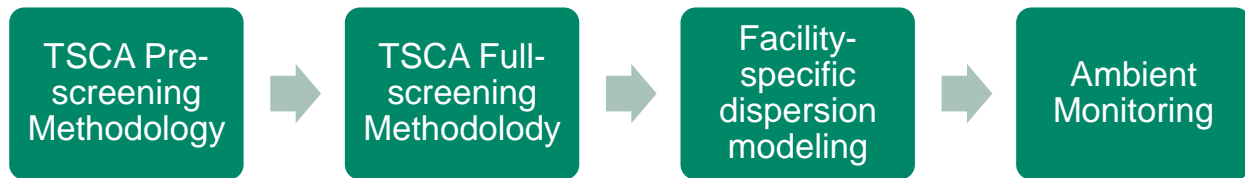
Figure 2: Proposed refinement of the tiered screening for industrial facilities (not for co-residential exposures)
