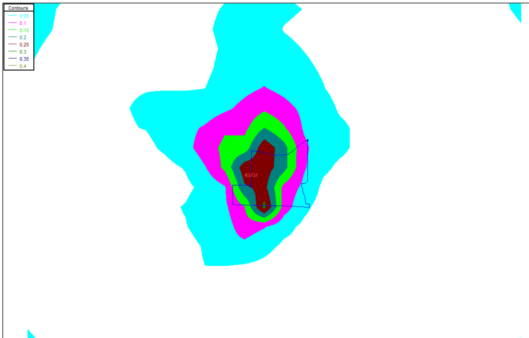
Figure A- 2 AERMOD Output Concentrations ( \mu\text{g m}^{-3} ) Contour Plot for Permit-style model for Year 2019
