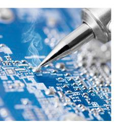
using copper salts and other plating chemicals. A solder mask (made of acrylic, polyurethane, or epoxy in combination with hardening agents and photoinitiators) is applied to insulate the copper and protect it from coming into contact with other materials. The solder mask is what gives PCBs their distinctive green color. Multiple layers can be constructed with epoxy laminate separating the layers.
