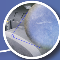
2019 GMC Sierra Denali lightweight carbon fiber composite truck bed includes pocket reinforcements made from recycled carbon fiber thermoplastic materials
