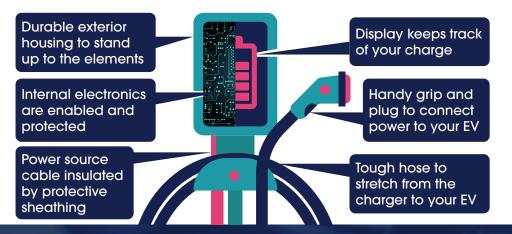
Plastic and other products of chemistry can be used for a wide array of components within the larger structure of alternative fueling stations and electric vehicle charging ports, such as charger housings, covers over front displays or touchscreens, lenses, connectors, light guides, and other components.
