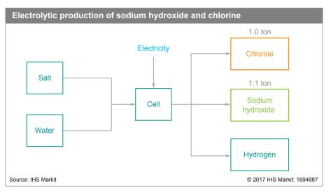
ECU. The figure illustrates the electrolytic process for making the co-products sodium hydroxide and chlorine.
